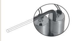
Simply tighten valves onto the manifold using a standard 3 mm. Allen hex wrench. (0.5 - 1 Nm. Do not over-tighten)
